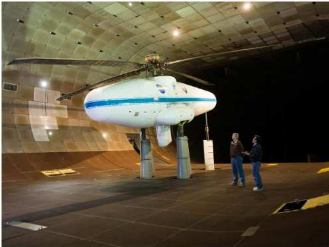
Figure 4.3: NASA's Large Rotor Test Apparatus (LRTA) fuselage.
