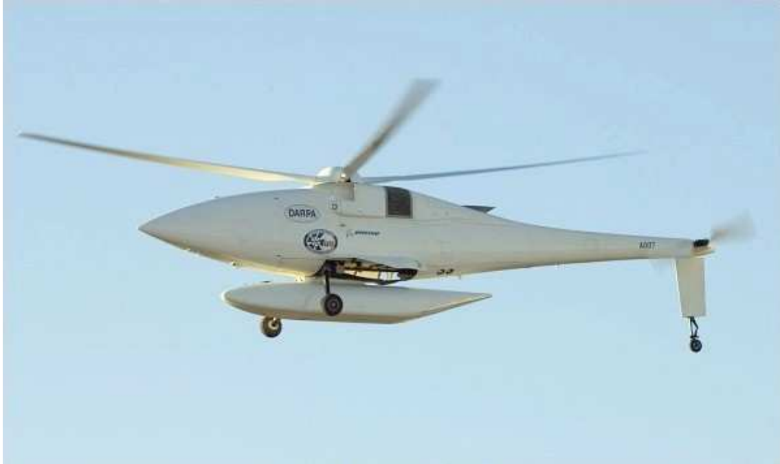
Figure 1.5: The Boeing A-160 Hummingbird used rotor speed variation (up to 60%) to achieve high endurance [11].
